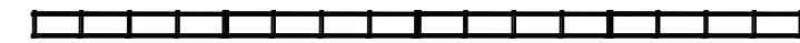
FIG 1. PLACE A ROW OF CONSTRUCTION FORMS ALONG DESIRED CHANNEL ALIGNMENT FOR FIRST FES LIFT.
