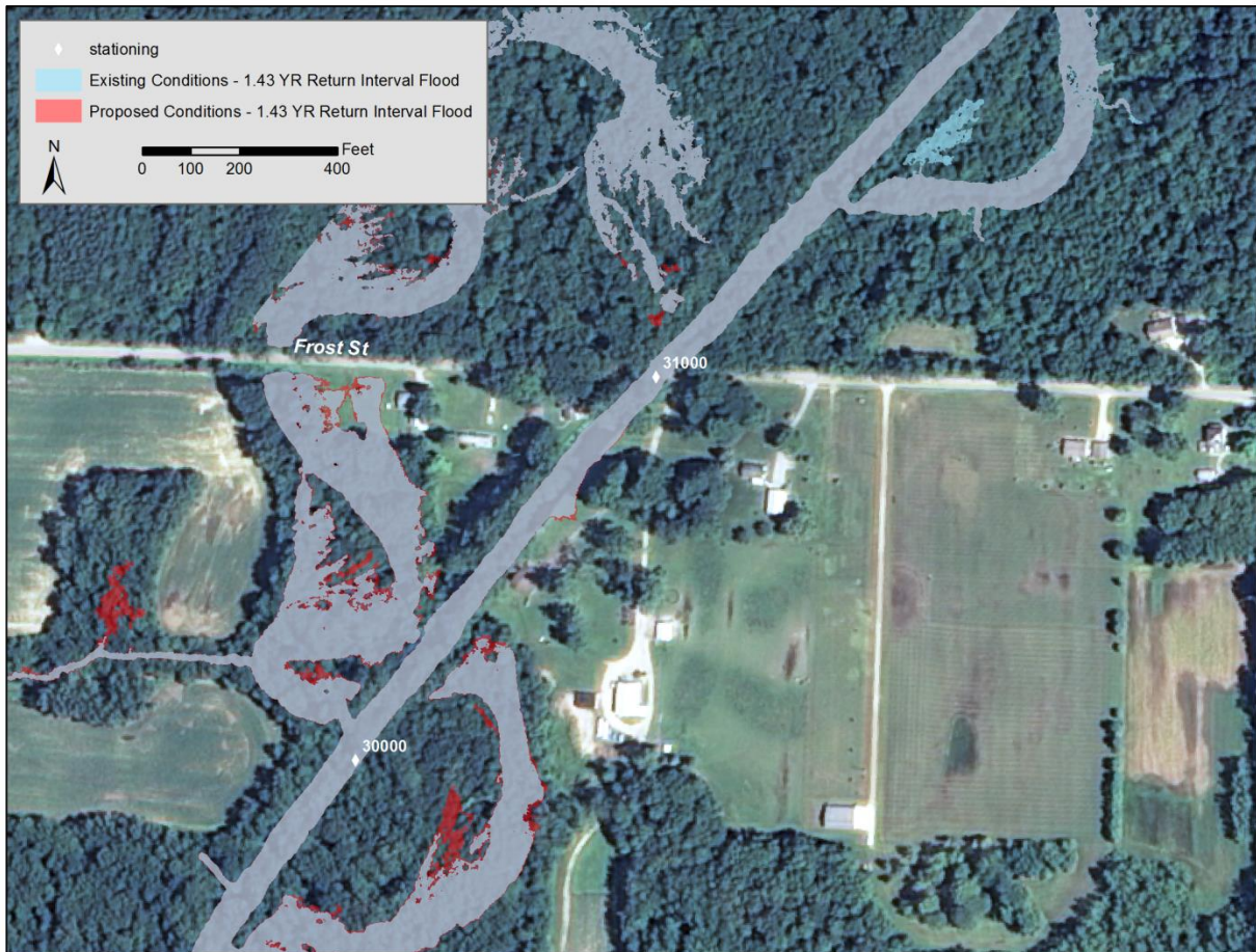
Figure 69. Plan view of the water surface extents around Frost St. at the 100-year flood quantile. The proposed (red polygon) water surface rises and covers a larger area than the existing (blue hatched polygon) area.
