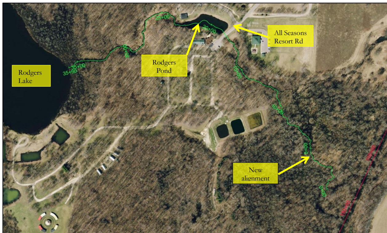
Figure 46. Location of the Rodgers Lake Outlet Channel and Pond. The channel will be re-aligned to its historic location. The current outlet to the Dowagiac River is at station 122+00.
