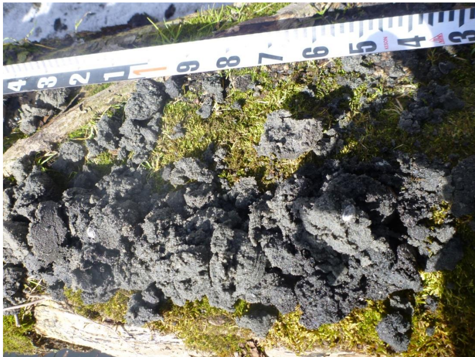
Figure 42. Sand within a DOR core at photo location 14. The sand is fine to coarse with bivalve shells throughout.
