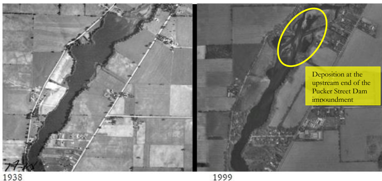
Figure 45. Comparison of the 1999 air photo and 1938 air photo at the Pucker Street Dam impoundment. A sizeable delta formed over the northern (top of figure) third of the reach.
