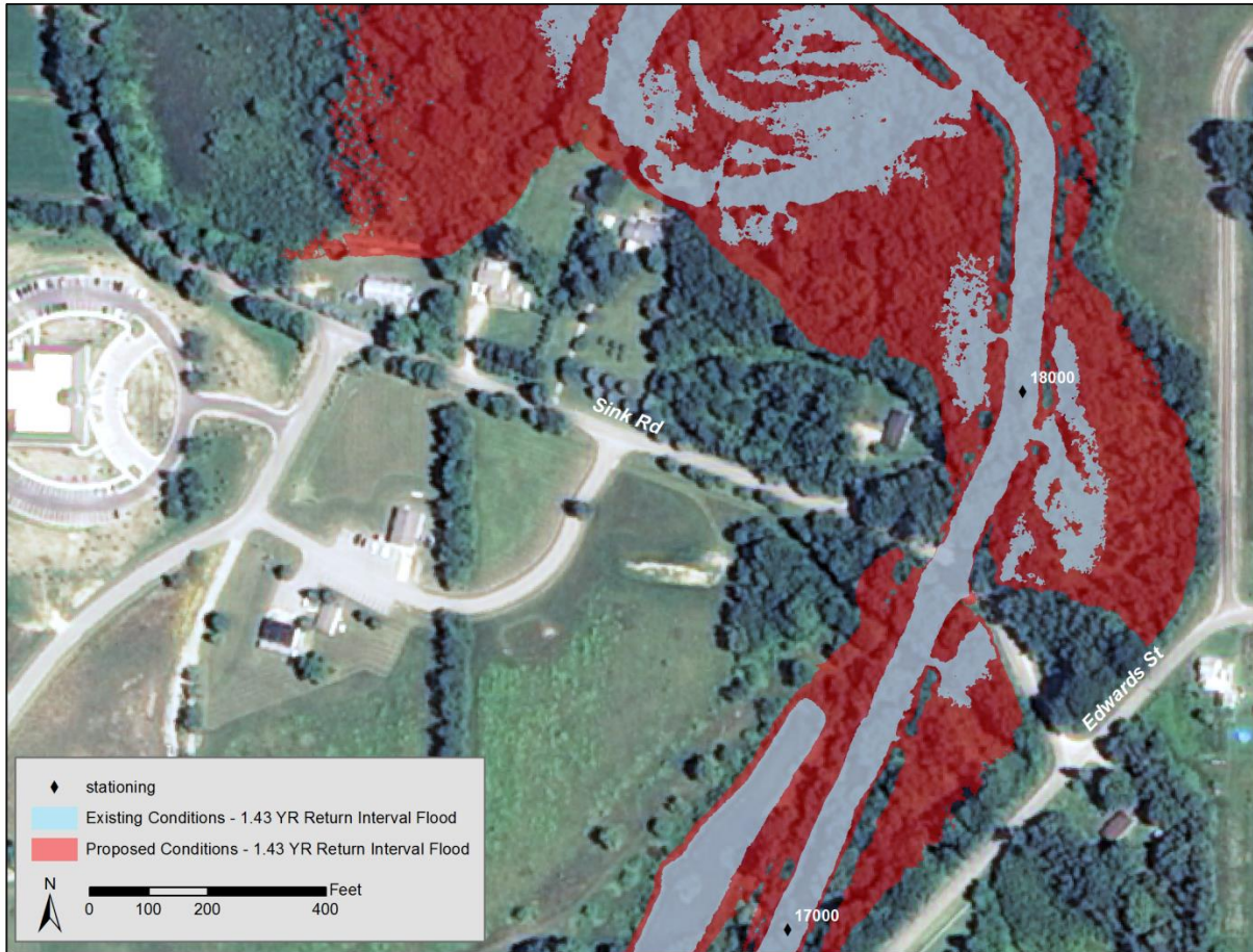
Figure 64. Plan view of the water surface extents around Sink Rd. at the 100-year flood. The proposed (red polygon) water surface rises and covers a larger area than the existing (blue hatched polygon) area.
